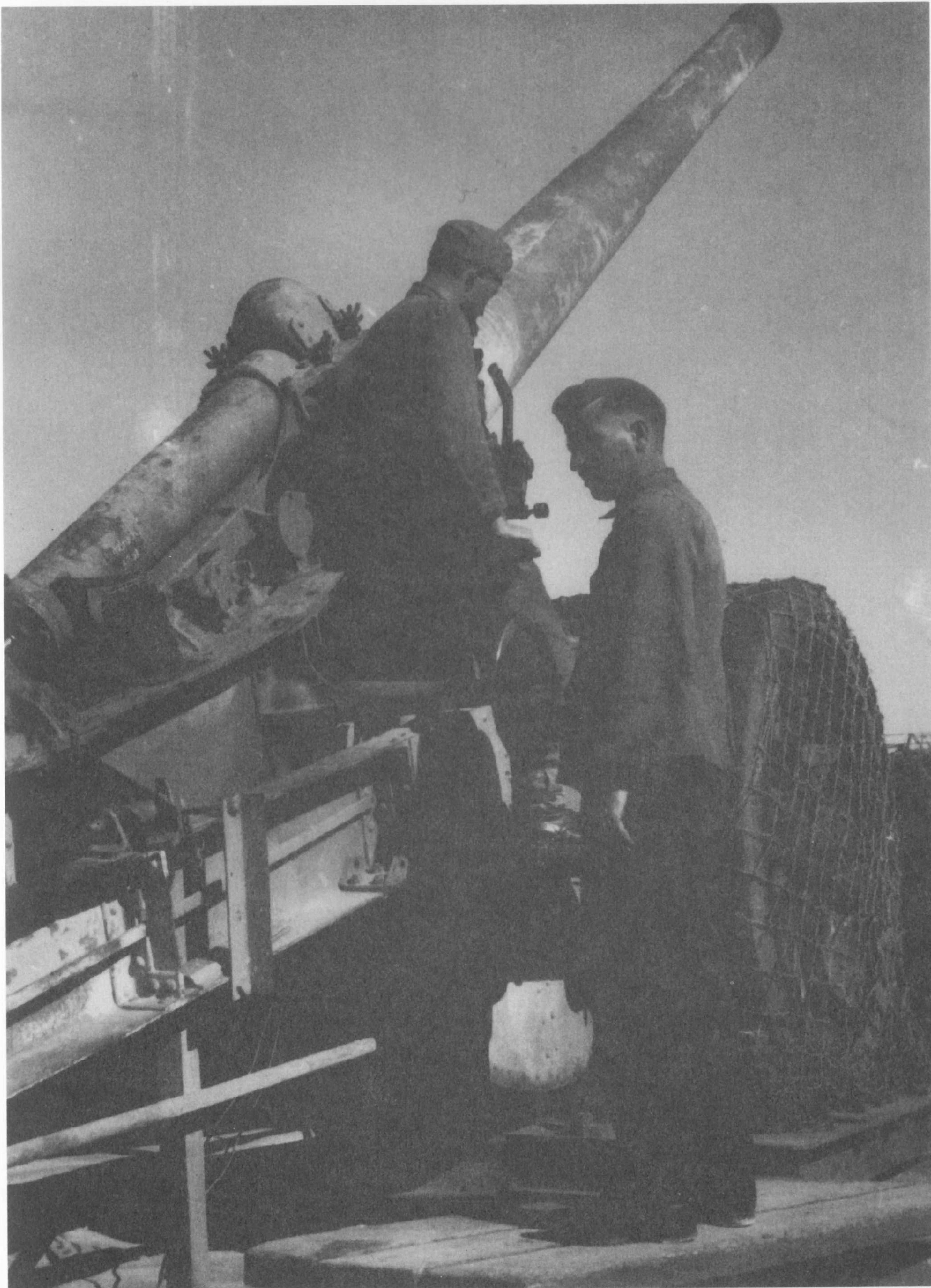
A 155mm Kanone 420 (f) of the Riva Bella Battery with its barrel at maximum elevation of +38 degrees. (BA)
