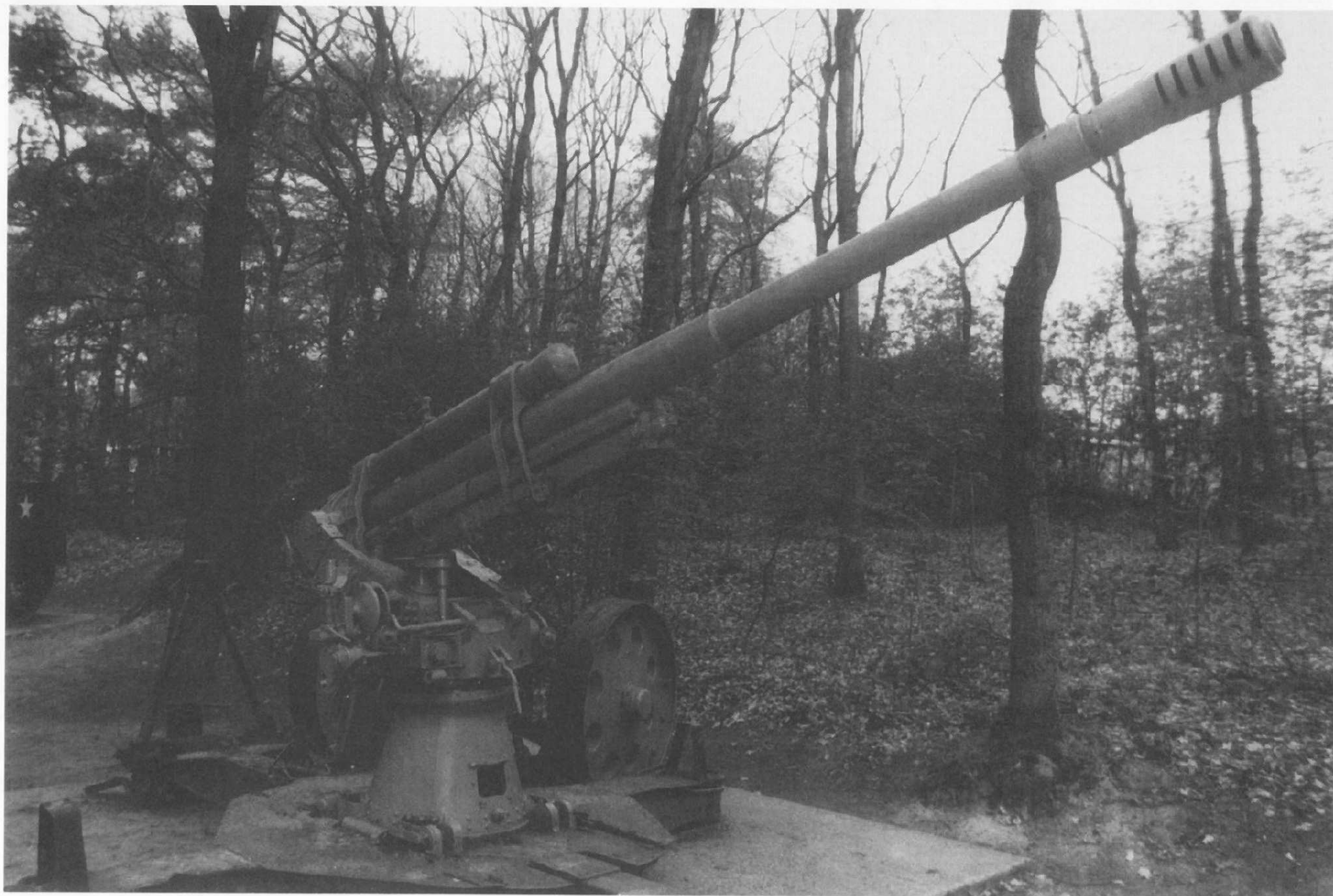
The 8.8 cm/8.5 cm Flak M 39 (r) in firing position. The rubber-tired iron wheels proved to be very robust and durable. With a barrel length of 4,693mm (55.2 calibers), the gun achieved a muzzle velocity of 800 m/sec and a maximum firing range of 15,500 meters. By comparison the German 88mm Flak 18/36 achieved a maximum firing range of only 14,800 meters. More than 1,000 Flak M39 (r) guns were used by the Wehrmacht.
