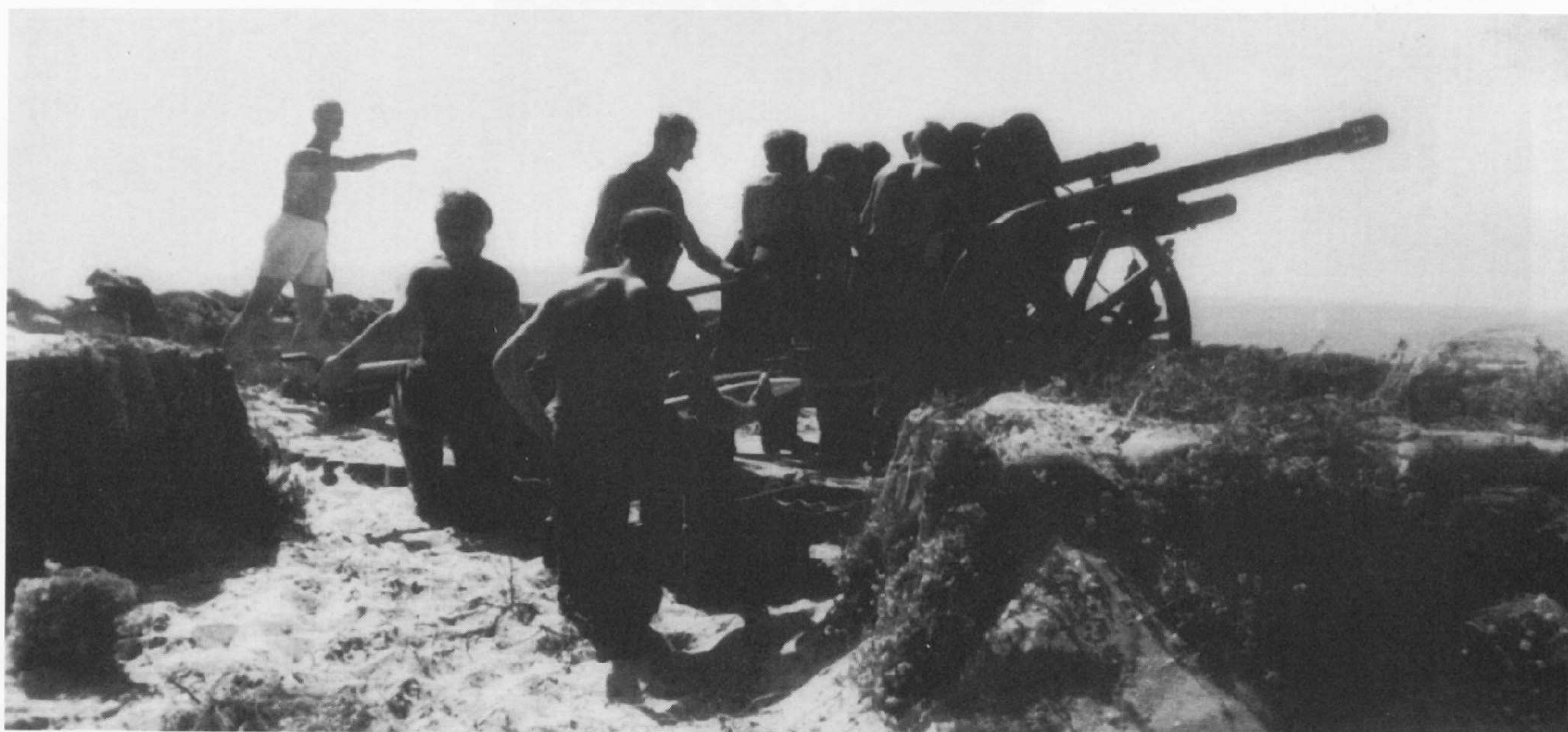
A 105mm Light Field Howitzer 18/42 in an improvised firing position on the Normandy coast. This cannon, which was built by Krupp, was one of the weapons most used by the army artillery on the invasion front.
